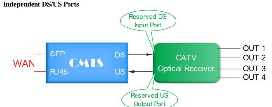
This mode is suitable for having optical receiver(or the light station) of reserving descending input port and uplink output port.
