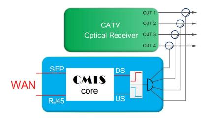
It's suitable to retain the original optical receiver, but there is no reserving upstream and downstream port.
